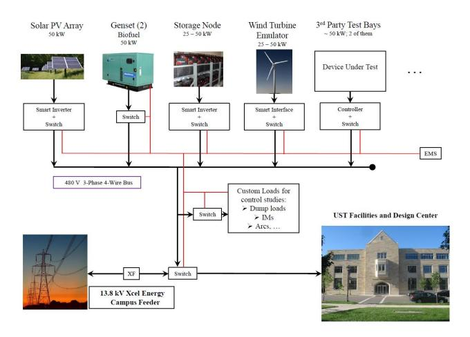
The detailed one-line diagram for the University of St. Thomas renewable Energy Facility (USTREF) is shown in the following two figures (below). Shown in the first figure are the system asset connections, switchgear, and protection. The second figure captures the hardware details of the portion of the microgrid that will be used to control the USTREF. These figures are necessary for the asset procurement process.
